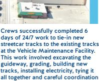
streetcar tracks to the existing tracks at the Vehicle Maintenance Facility. This work involved excavating the guideway, grading, building new tracks, installing electricity, tying it all together and careful coordination with streetcar operations. This is the first time the existing system was connected to new tracks!
